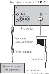
Of the two lead wires connected to the back lamp, connect the one in which the voltage changes when the gear shift is in the REVERSE (R) position. This connection enables the unit to sense whether the car is moving forwards or backwards.
