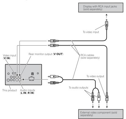
It is necessary to change AV Input in System Menu when connecting the external video component.
